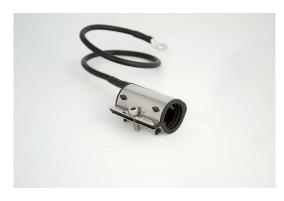
The grounding clamp for 7 mm coax cables such as AIRCELL 7, ECOFLEX 7 etc. is used to eliminate potential differences (voltages) between the coax cable and the earth potential, which can occur, for example, during a thunderstorm. The grounding clamp has a solid stainless steel housing with a hinge and thus a compact structure. Installation is fast and easy because there are no loose parts and the earthing clamp can be closed with just one screw. No extra taping is needed.
