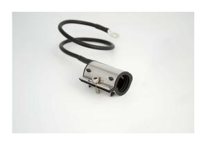
The grounding clamp for 10 mm coax cables such as Ecoflex 10, Aircom Premium etc. is used to eliminate potential differences (voltages) between the coax cable and the earth potential, which can occur, for example, during a thunderstorm. The grounding clamp has a solid stainless steel housing with a hinge and thus a compact structure. Installation is fast and easy because there are no loose parts and the earthing clamp can be closed with just one screw. No extra taping is needed.
