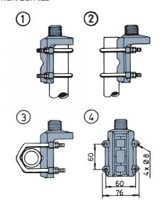
2 Mast tube  $D_0$ , max = 54 mm Mast tube  $D_0$ , min = 16 mm
