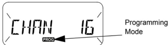
In 'Programming Mode', the radio is capable of setting values for each channel by toggling between the different programming modes available:
