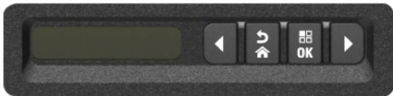
**Figure 5:** Charger Display and Keypad
