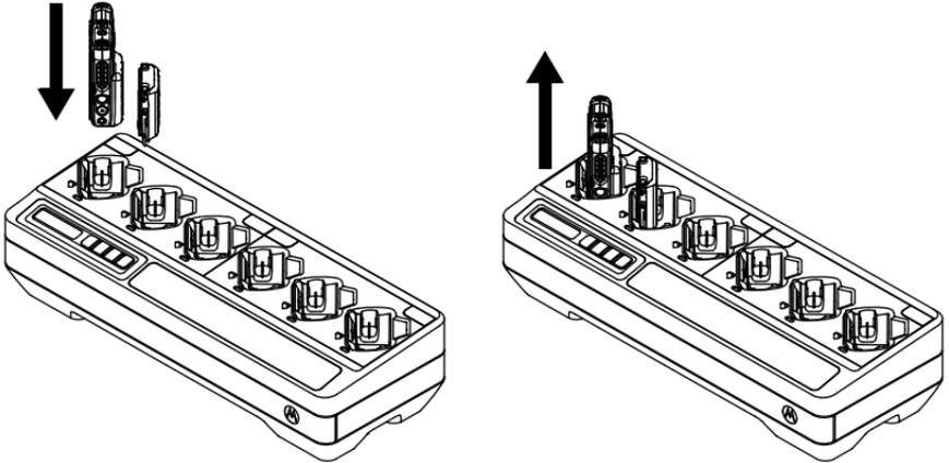
**Figure 4: PMPN4380\_ Charging Procedure**
