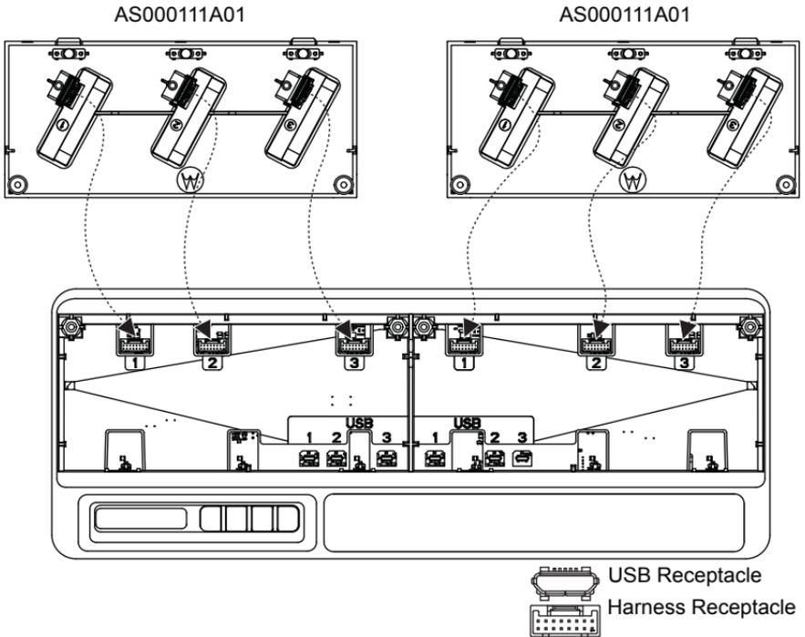
**Figure 28:** Securing AS000111A01 Charging Pockets to Multi-Unit Charger Base
