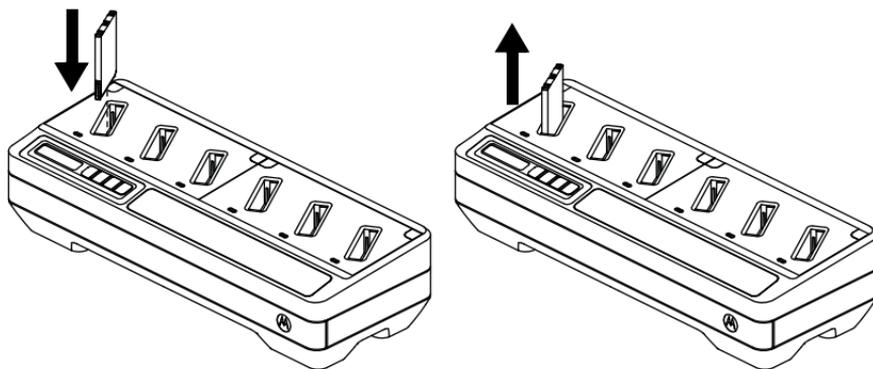
**Figure 3:** PMPN4370\_ Charging Procedure
