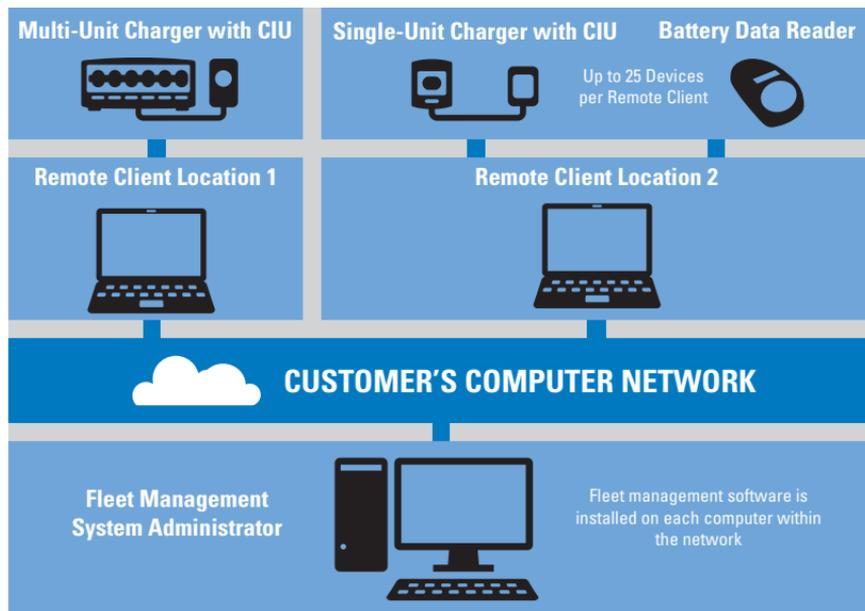
**Figure 20:** IMPRES Battery Management via Network Chargers
