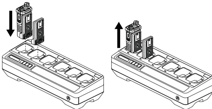
**Figure 2:** PMPN4283\_/PMPN4286\_/PMPN4288\_ Charging Procedure
