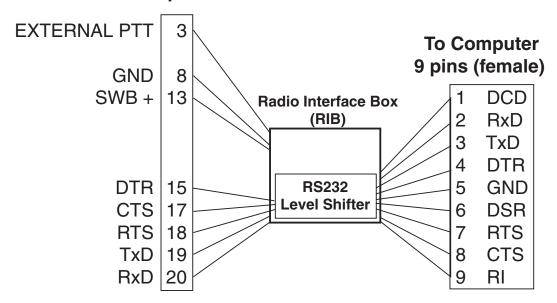
**Note:** If the Active Data Cable shall be used in conjunction with any other accessory using PTT functionality (EXTERNAL\_PTT), the black colored cable at the accessory connector of the Active Data Cable must be removed and cut.
