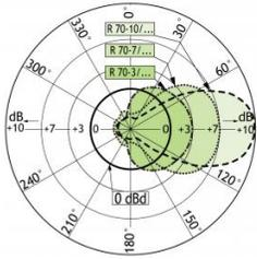
If the antennas are mounted for vertical polarization, these curves show the radiation patterns in the horizontal plane (horizontal coverage).
