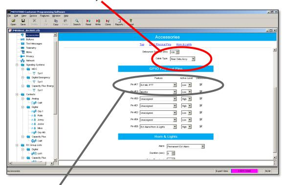
To use the external microphone you also need to set: GPIO Pin #17 to Ext Mic PTT, active Low.
