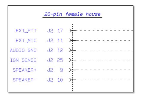
Recommended connectors for ignition sense, microphone and speaker
